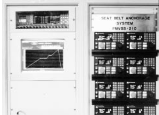
Fig. 4 Front panel of the anchorage test system
