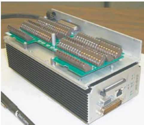
DAQ750 shown with cover removed
